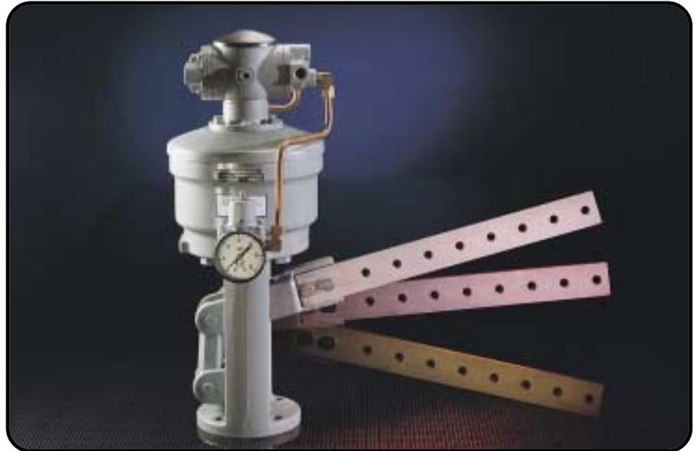
Conoflow's Pneumatic Lever Actuators are rugged and powerful units used to automatically position dampers, louvers, variable pitch fans and to make various mechanical adjustments to process machinery. Low profile (only 18" high) requires less headroom. A sturdy ductile iron yoke with large mounting base provides rigid mounting. The steel lever arm has eight take-off positions for stroke flexibility.
