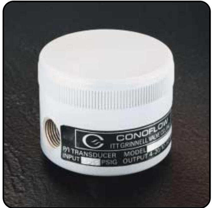
Conoflow's Model GPT82 Pressure to Current Transducer simplifies the monitoring of control loop systems by converting a pneumatic signal to a proportional current output. The compact, lightweight design affords easy line mounting installation into a 2-wire instrument loop. An optional wall mounting bracket is available.
