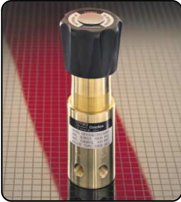
The Conoflow HP300 High Pressure Regulator is designed to accurately control supply pressures up to 10,000 PSIG (69 MPa). This piston sensing, self-relieving regulator allows pressure setting reduction in a closed system by relieving downstream pressure through the regulator.
